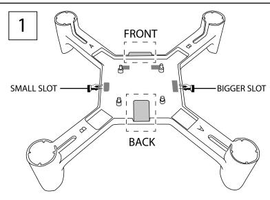
Pay close attention to the orientation of the drone frame. Note that the front has a small tab sticking out and the back has a small recess.
